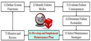
[Fig.5: Planning Process for Reliability-Centered Maintenance (RCM)]
