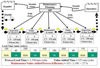
[Fig.9: Maintenance Value Stream Mapping (Before Improvement)]
