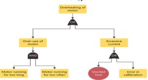
[Fig.11: Fault Tree Analysis (FTA) for Overheating of the Motor]
