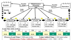
[Fig.18: Maintenance Value Stream Mapping (after Improvement)]
