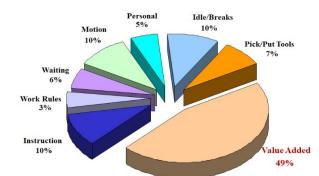
[Fig.19: Shutdown Waste Time Analysis (after Improvement)]
