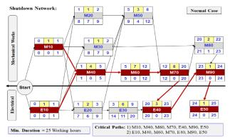
[Fig.8: Shutdown Project Network for Normal Case (Before Improvement)]
